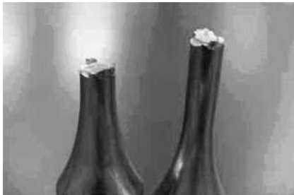
Fig. 2 SAE 4340 steel test specimen with AC-HVAF applied, 0.003 in. thick WC-Co coating following fatigue testing at 220 ksi
